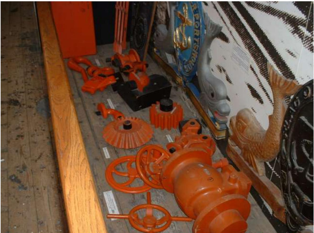
the core box. Core prints, to show where the casting was hollow, were just varnished wood. Core boxes were also varnished wood, the core channels picked out in black. M. C. D.
